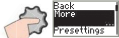
Select More to go to next level: - basic settings - all settings - diagnostics
