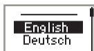
Select your language before entering the first LCD-menu. Available for the first 30 seconds after power-on of the sensor.
