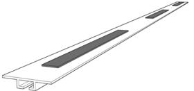
Ensure that all pieces of the retainer are installed straight, preferably by using a level.
