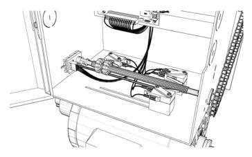
5. Attach the red spaded wire to the "Fully Closed" limit switch's available spade terminal.
