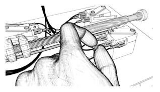
6. Attach the green spaded wire to the "Fully Open" limit switch's available spade terminal.
