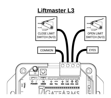
The L3 does not support monitored safety eyes. Thus the default configuration should work as expected.
