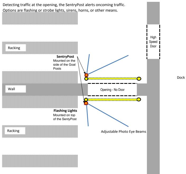
Once any of the 4 beams detect vehicles, or pedestrians, both flashing lights will be active until detection ceases.
