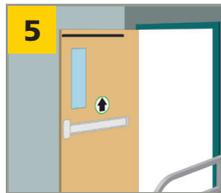
Align the housing with the top of the door at the chosen location (ensuring proper orientation) and then mark the mounting holes at both ends. *Avoid mounting holes near door seams.* Also mark the appropriate end for a wire-passage function hole (if required). This hole may be no more than 1" in diameter.
