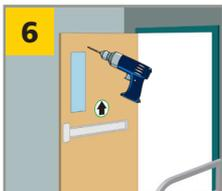
Drill the marked holes (ensuring proper hole size).
