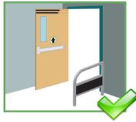
Choose a location that does not interfere with door hardware (e.g. finger guards, lock rods, etc.).
