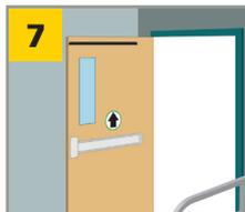
Align the housing with the pilot holes and secure to the door with the 2 provided screws.
