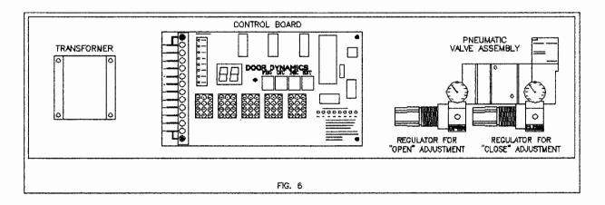
The door speed pressure settings have been factory preset to 35 PSI for the closing cycle and 40 PSI for the opening cycle.
